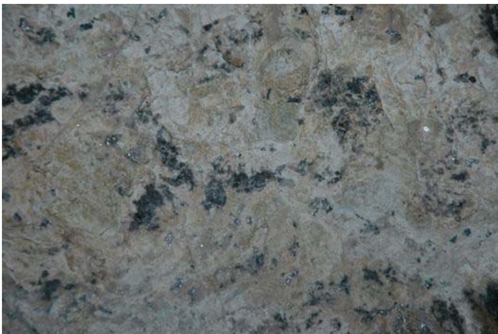
Figure 11-1 Recrystallised pink feroan dolomite of the lower metre of the RSC, showing the abundance of visible shiny crystals of carrollite (Co 2 CuS 4 )
